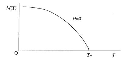
For a ferromagnetic material in the absence of an applied field (H=0), the spontaneous magnetization is a maximum at T=0, decreases to zero at the critical temperature  $T = T_C$ , and is zero for all  $T > T_C$ . For temperatures just below  $T_C$  the magnetic susceptibility and the temperature coefficient of M might be modeled by the expressions
